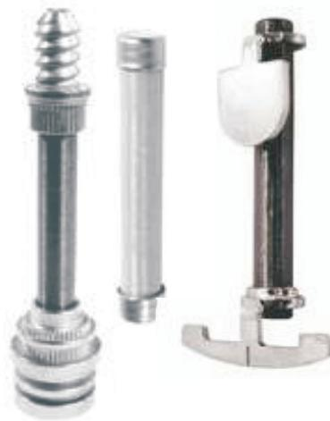
The resistor element is a resistive wire, which is wound in a single layer on a fiberglass core. Metallic caps or electrodes are fixed to the ends of the resistive core, following the specific ignition system characteristics. A coating protects the resistive element against moisture and mechanical shock, plus is able to withstand high temperatures. These products can be molded with epoxy resin, thermoplastic or thermo set materials.
